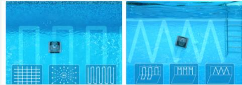
Connected to the Wybot app, the user can access predefined movement paths for the ground (3 patterns) and the walls (3 patterns).
